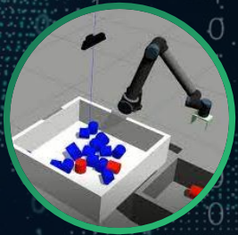
Example: Computer-vision based bin picking
